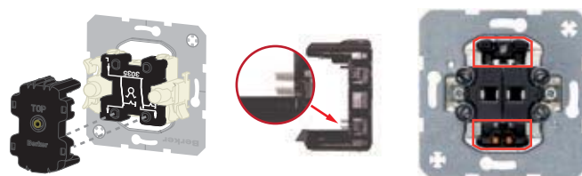
Figure 5: The LED unit has contact springs (s. figure in the middle), which ensure simple snapping-on from behind
